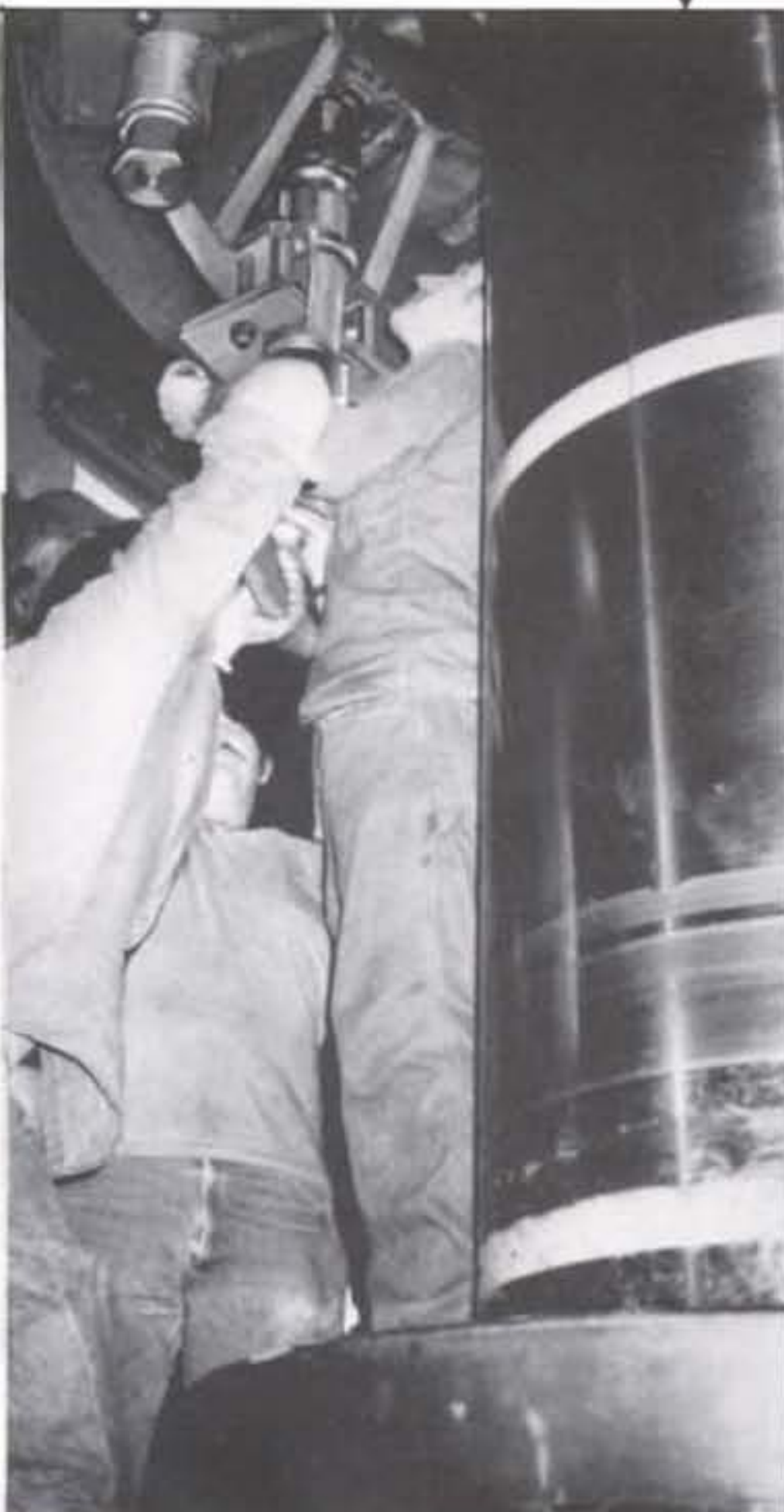
Adjusting a Kingsbury Type Thrust Bearing to equalize the thrust load on all shoes. ▼
