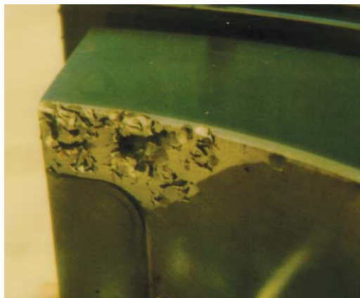
Figure 29 Eroded Babbitt From Spragging
