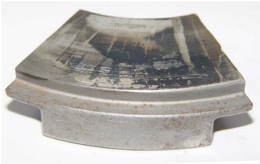
Figure 20 Outer Edge Babbitt Erosion
