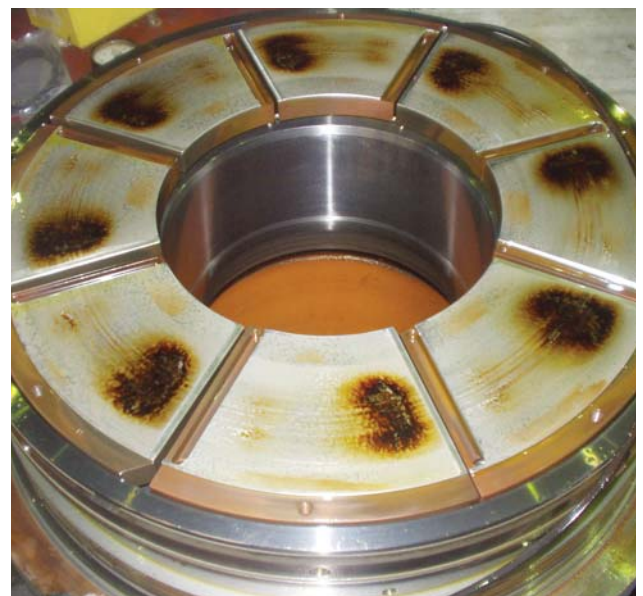
Figure 18 Overheating, Oil Additives Plated Out
