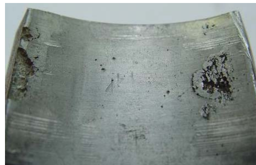
Figure 30 Spragging Effects On Pad
