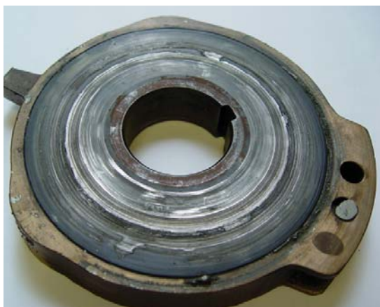
Figure 21 Oil Circulator Fused To Collar
