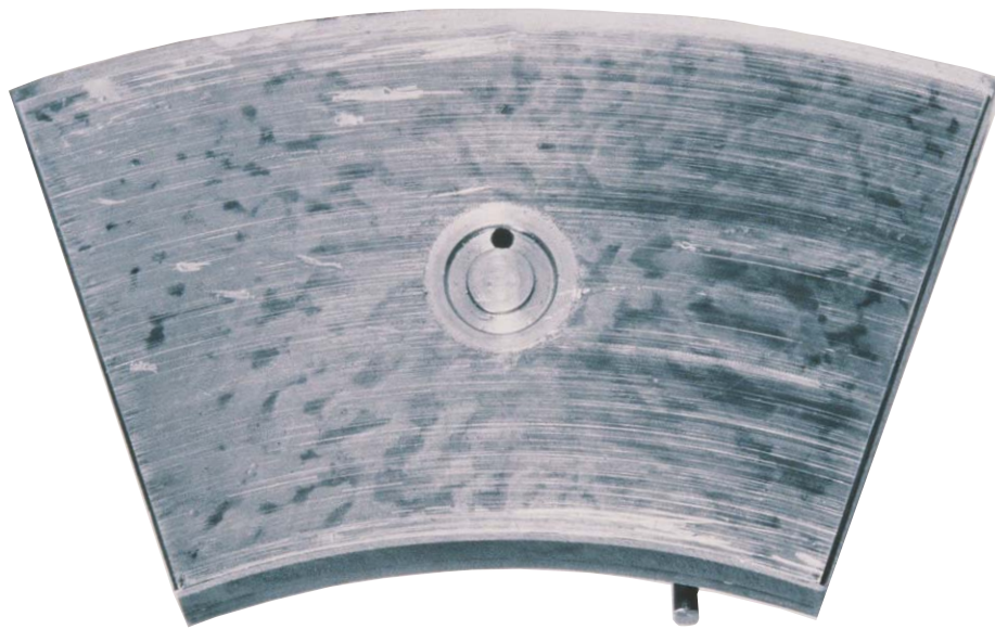
Figure 15 Thrust Shoe Surface Abrasion
