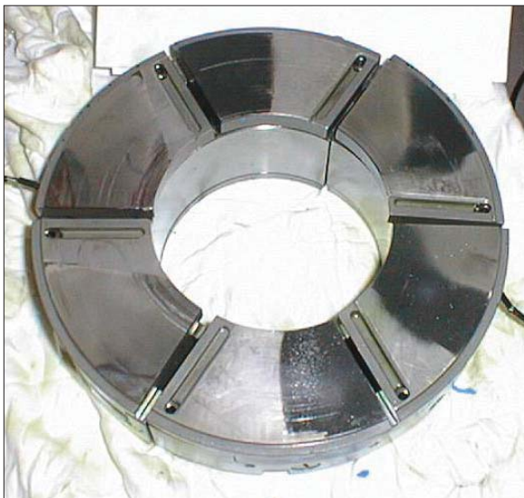
Figure 34 Example of Bearing Corrosion
