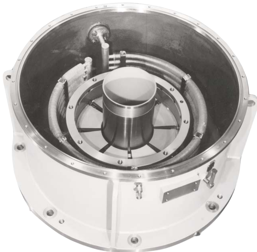
Figure 14 Vertical Thrust Bearing Oil Sump and Cooling Coils
