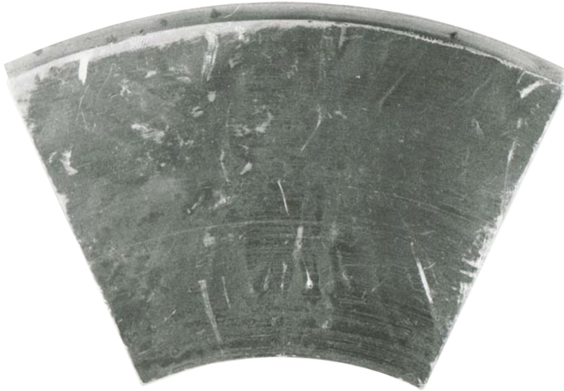
Figure 16 Tin Oxide Damage
