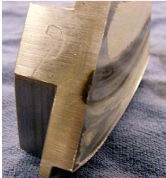
Figure 19 Tilting Pad Showing Complete Babbitt Removal
