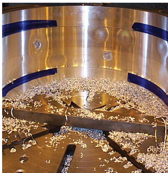
Figure 23 Large Hydrogen Blisters
