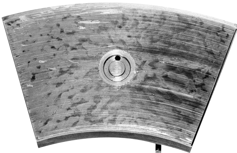
Figure 2. Thrust Shoe Surface Abrasion
