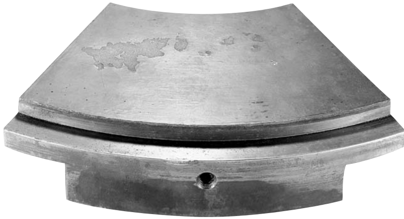
Figure 3. Tin Oxide Damage
