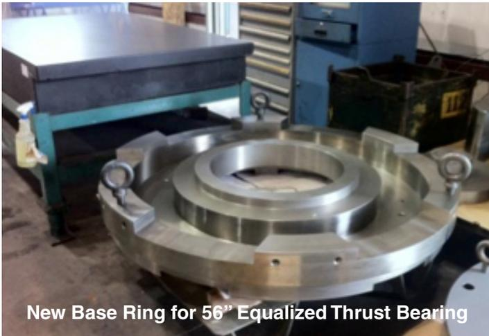
**New Base Ring for 56" Equalized Thrust Bearing**
