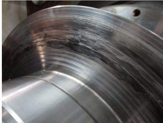
FIGURE 6. Damaged thrust collar from April 2017
