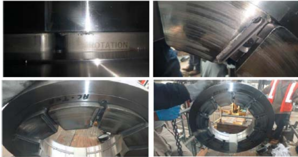
FIGURE 2. Thrust bearing damage discovered during DGS replacement in July 2015
