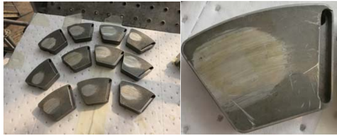
FIGURE 7. Active thrust pads removed in July 2018 (close up on right)
