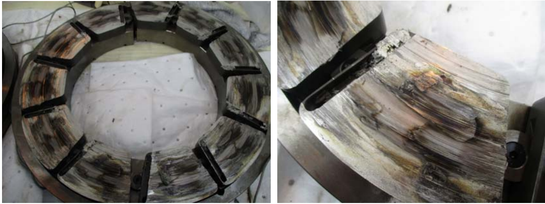
FIGURE 5. Failed active thrust bearing from April 2017 (close up on the right)
