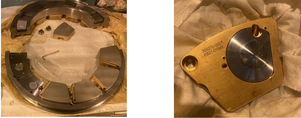
FIGURE 19. New thrust bearing (active side only) prior to installation in 2022
