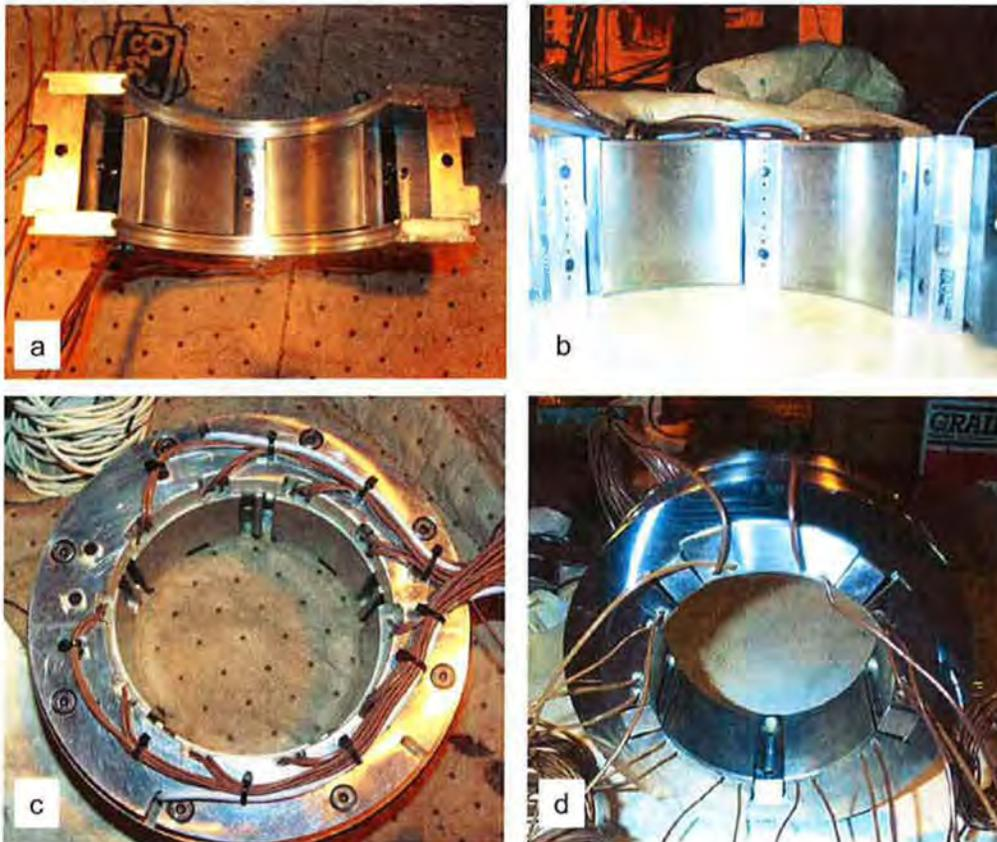
Figure 4. Test bearings: a) conventional with laby seals, b) spray nozzle, c) LEG<sub>®</sub>, d) BPG<sub>®</sub>.
