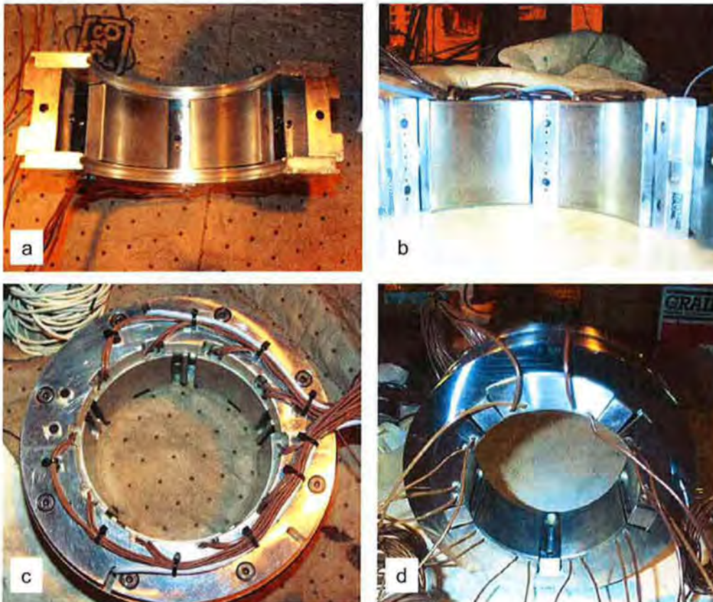
Figure 4. Test bearings: a) conventional with laby seals, b) spray nozzle, c) LEG ® , d) BPG ® .
